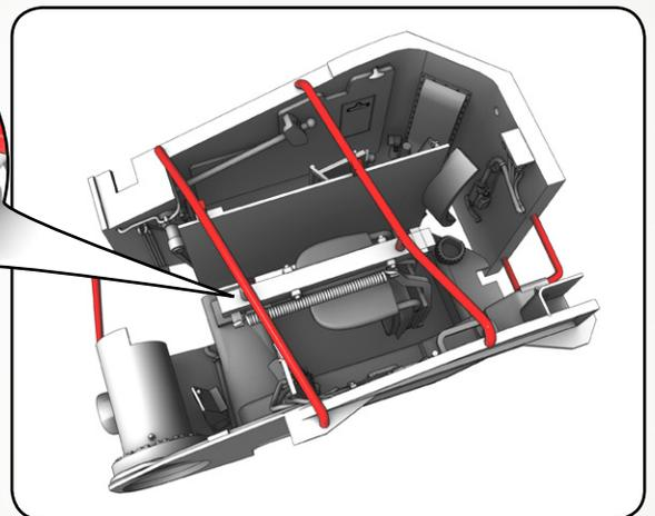
Please cut the red parts of, to remove parts from frame.
